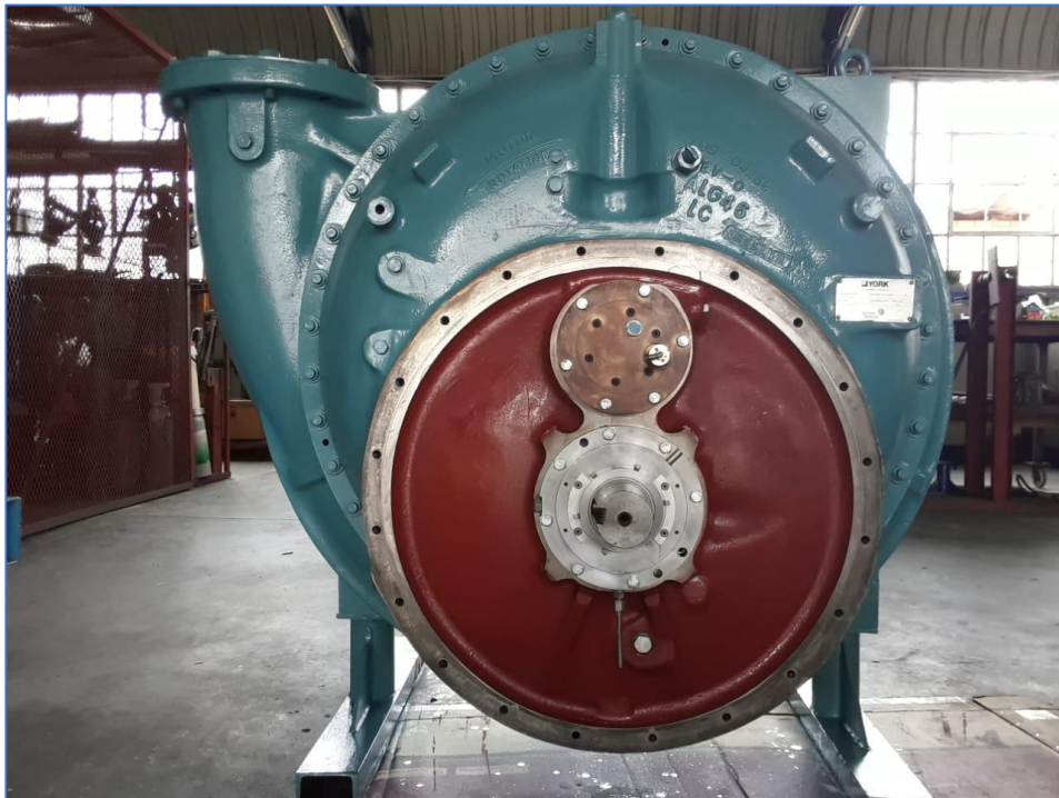
York YK J4 Compressor Float inspection
