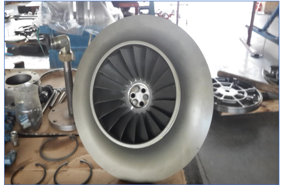
Disassembly York YK J4 Compressor
