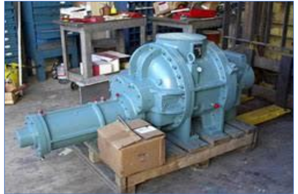
Frick TDSH 233 Ammonia Compressor
