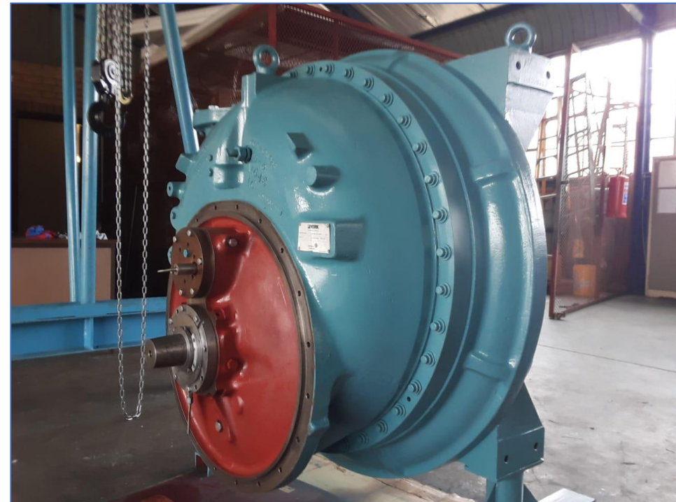
Disassembly York YK J4 Compressor
